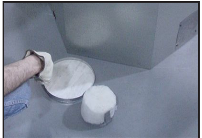
Figure 9.11 Discard the seal cap, remove and discard the insulation basket. Note: Once the seal cap has been removed it CANNOT be reattached.
